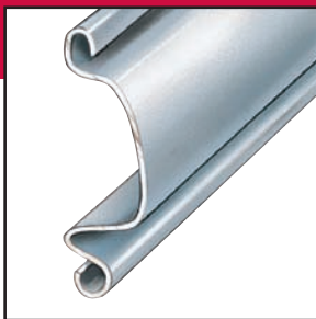
No. 4 —Curved-faced single crown slat available in up to 18-gauge steel or stainless steel. Depth of crown: \frac{1}{8} ", 2\frac{1}{8} " on centers.
